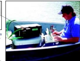
The 10-AU configured with the 25 mm One-Piece Flow Cell, a garden hose, and a 12 VDC cable for continuous field operation.
