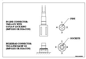
Figure 1. WETStar bulkhead connector
