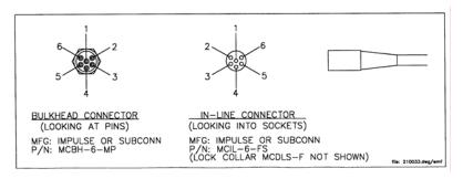
Figure 2. Optional 6-pin digital WETStar connector
