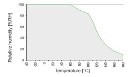
The grey area shows the allowed measurement range for the humidity sensor.
