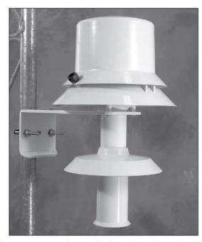
radiation errors. Compact shield components reduce radiation-absorption and improve aspiration efficiency. Specially selected plastic materials provide high reflectivity, low conductivity, and maximum weatherability.
