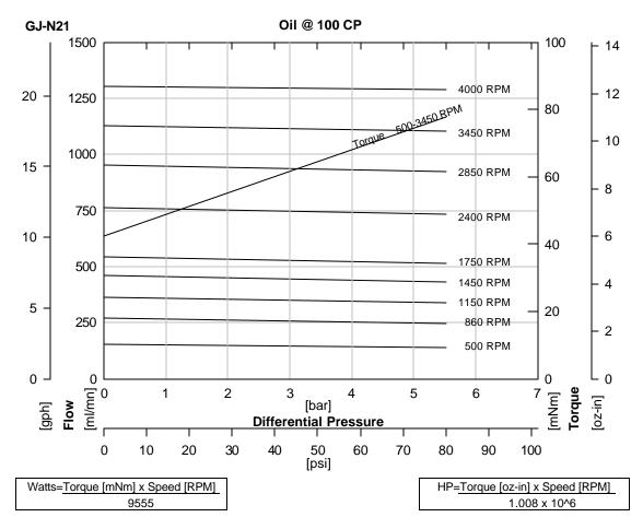
To calculate torque, multiply correction factor by torque from viscosity curve above.
