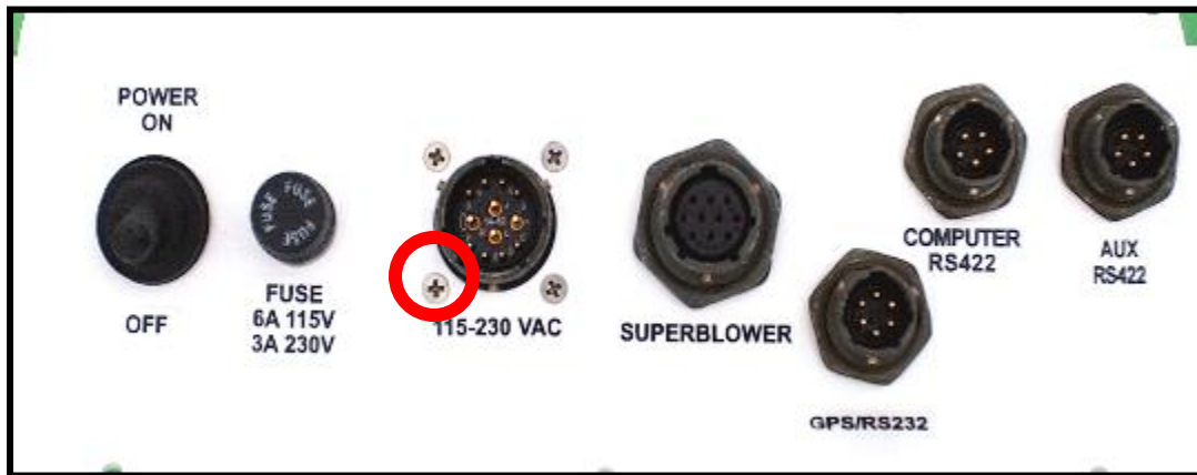
Figure 6-8. Ground metal on Front Connector Panel
