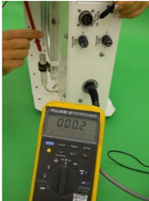
Figure 6-7. Test and reading for Ground continuity
