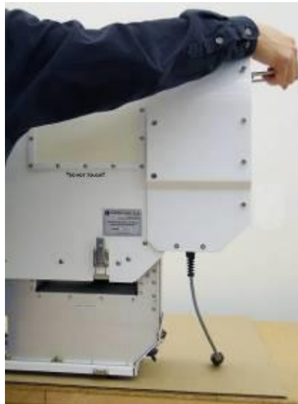
Figure F-2. One person, lifting the radiometer hood straight up
