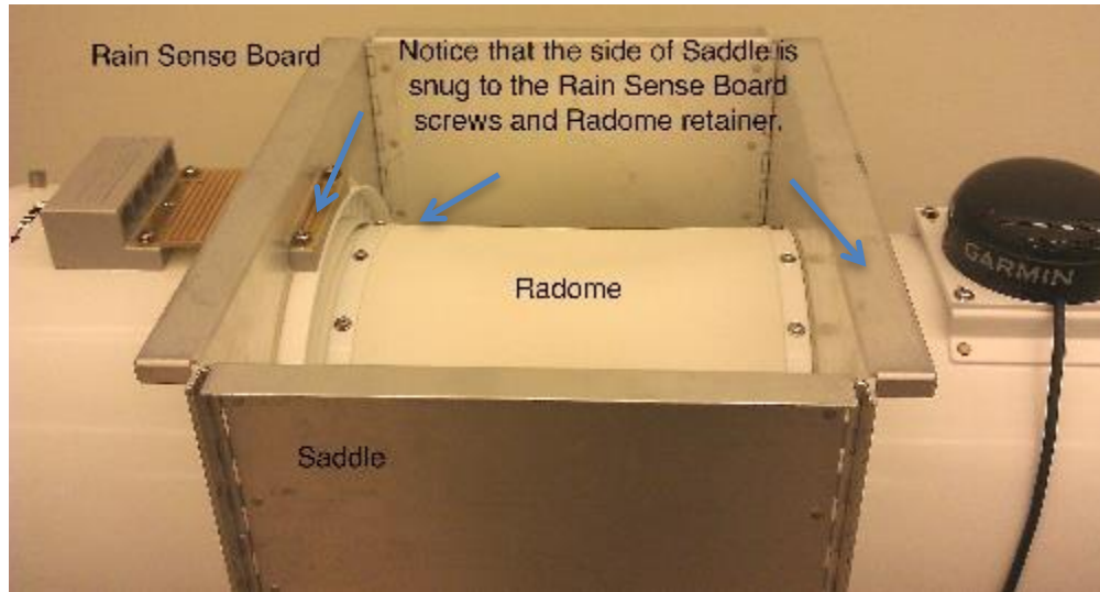
Figure C-3. Saddle for Cryogenic Target, properly seated
