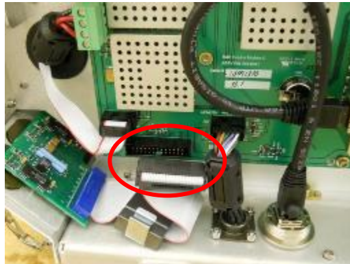
Figure F-17. Ribbon connector unplugged from the MCM board
