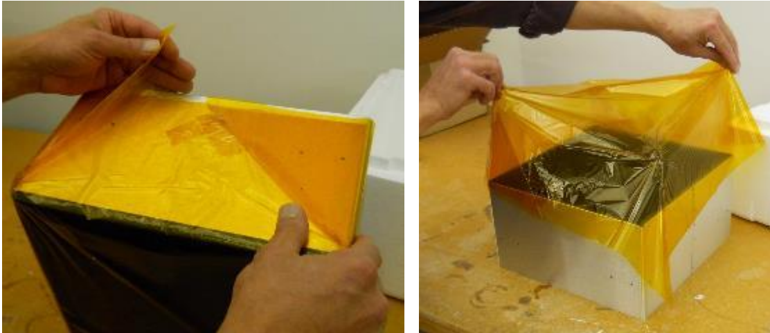
Figure C-8. Untaping and removing protective liner
