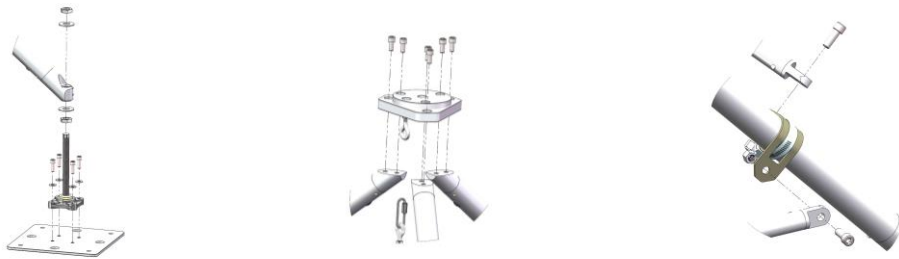
Figure A-3. EZ-Tripod Assembly Components. Cross Strut, Top Plate, and ESA (exploded views)
