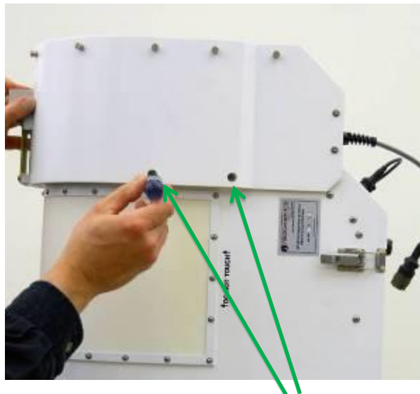
Figure F-27. Removing Superblower screws (two on each side)
