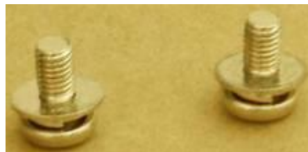
Figure F-20. Screw – lock washer–flat washer combination
