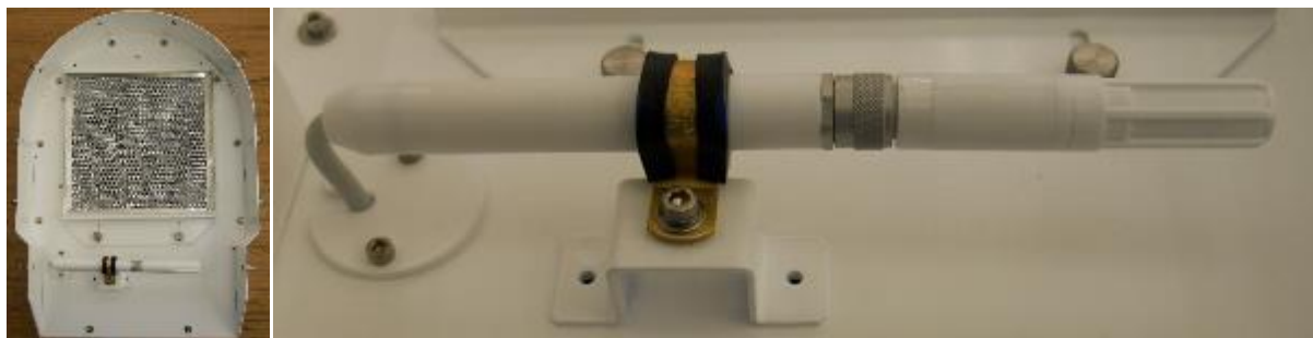
Figure C-18. Superblower with End Cover removed; sensor and filter
