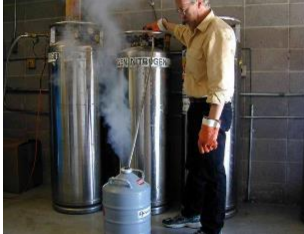
Figure C-15. Dewars used for storing and handling LN2
