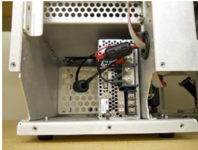
Figure F-19. Front of Power Supply, showing two connection shields
