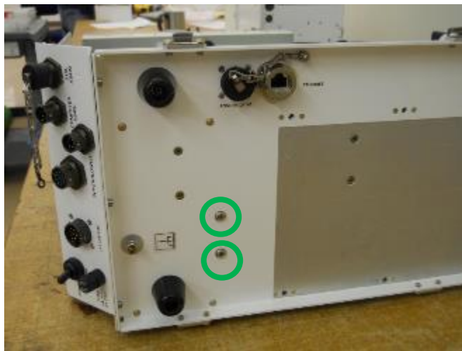
Figure F-14. Underside of radiometer, AC Line Filter retaining screws circled
