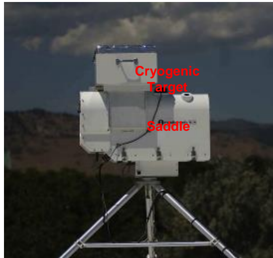
Figure C-2. Radiometer with Saddle and Cryogenic Target in place
