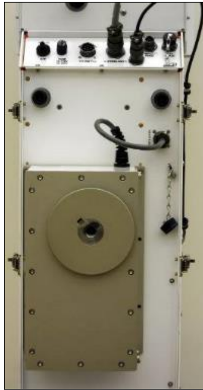
Figure G-2. Underside of radiometer with Azimuth Drive installed
