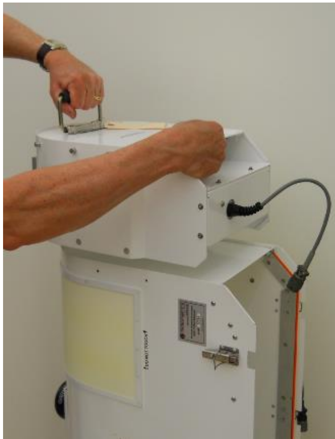
Figure F-28. Lifting Superblower away from the radiometer hood
