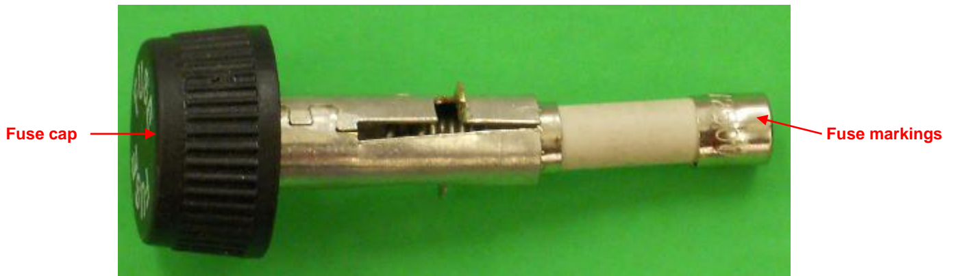
Figure F-30. Fuse in fuse cap, markings visible
