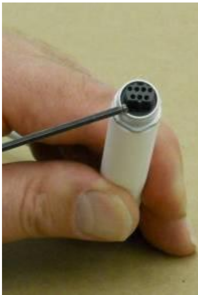
Figure F-24. HC2-S3 Ambient Air Probe, showing receptors
