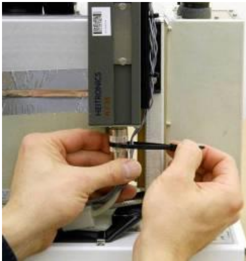
Figure F-8. Fastening thermal sensor cable pairs with cable-tie retainers
