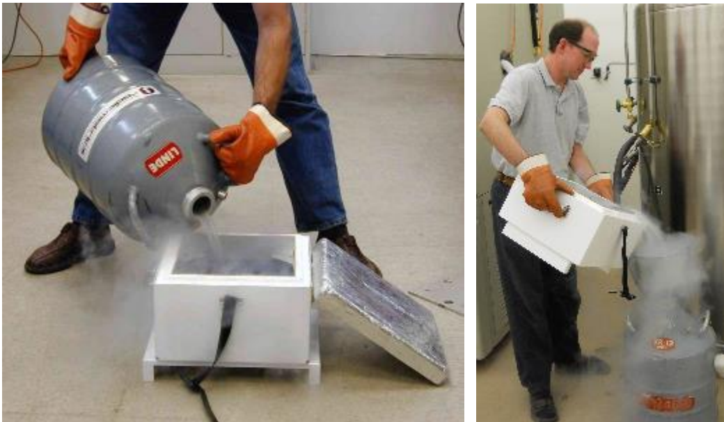
Figure C-16. Handling LN2: Filling Cryogenic Target (left) Pouring residual LN2 into Dewar after calibration is finished (right)
