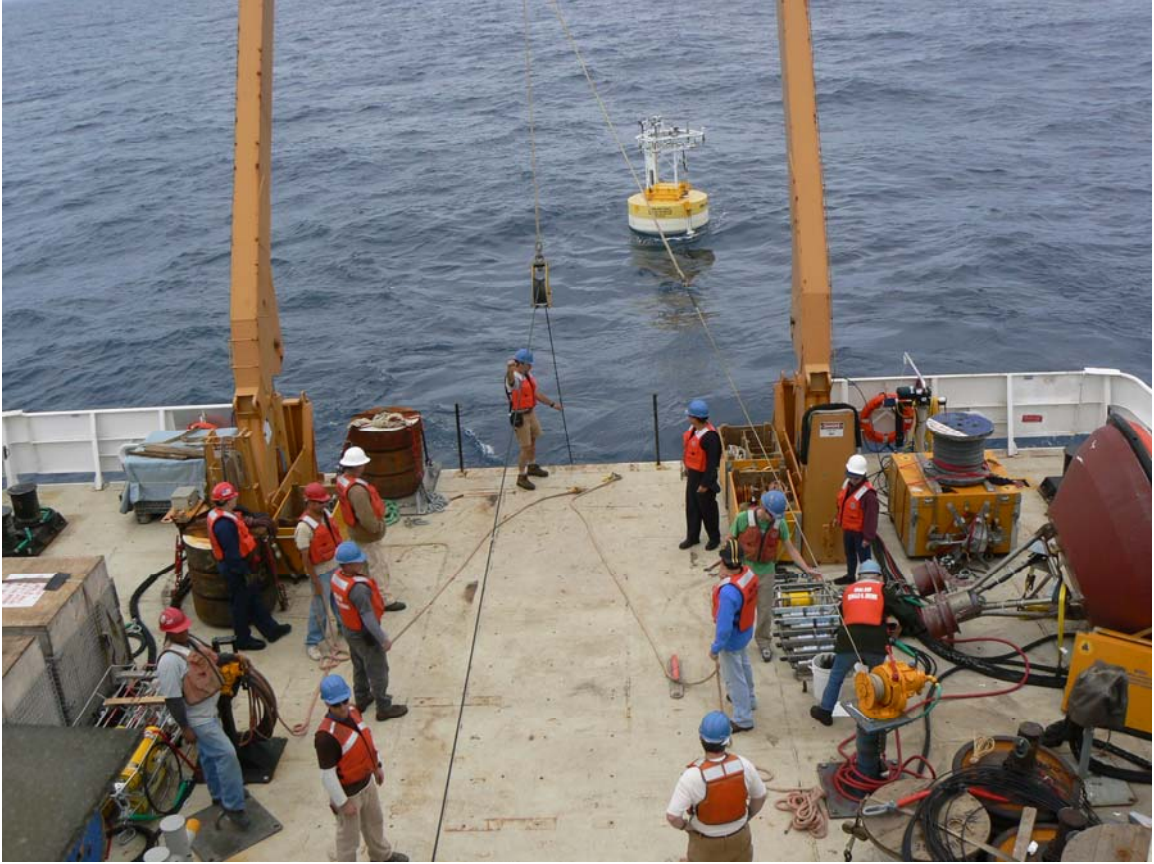
Figure 10. Photograph of WHOI buoy shortly after being placed in the water but prior to placement of subsurface sensors (aft deck of the Ronald H. Brown).
