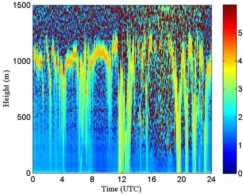
Figure 4. Time-height cross section of ceilometer backscatter intensity for October 29.
