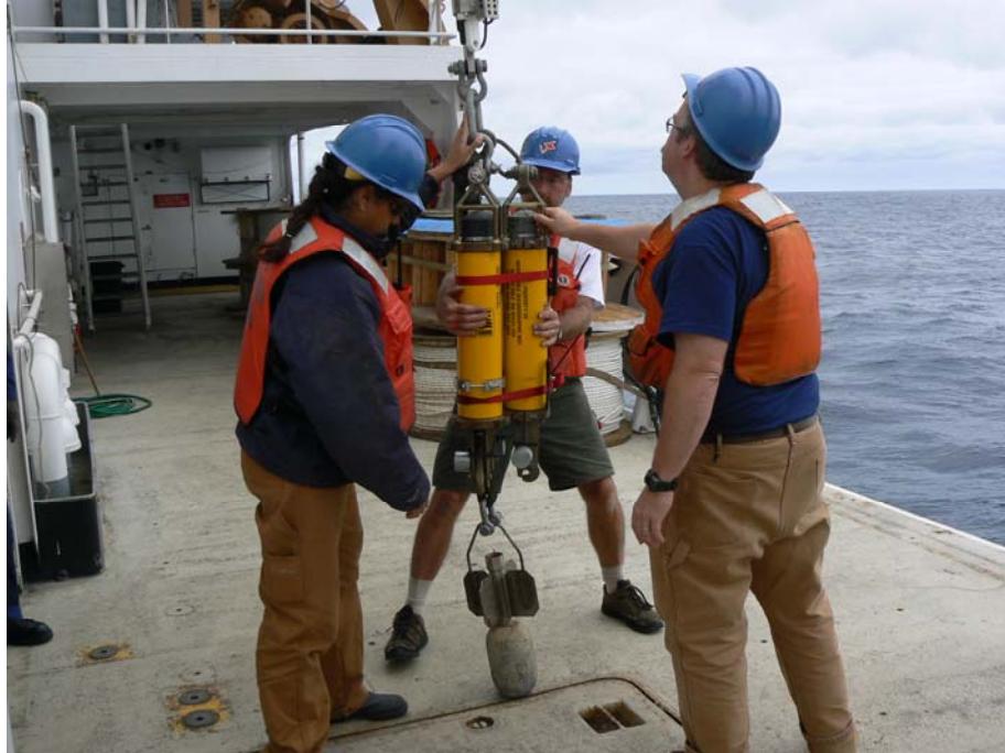
Figure 11. Photograph of CTD just before deployment at 20 S 75 W (L to R: Dana Mancinelli, Jeff Lord, Robert Weller).
