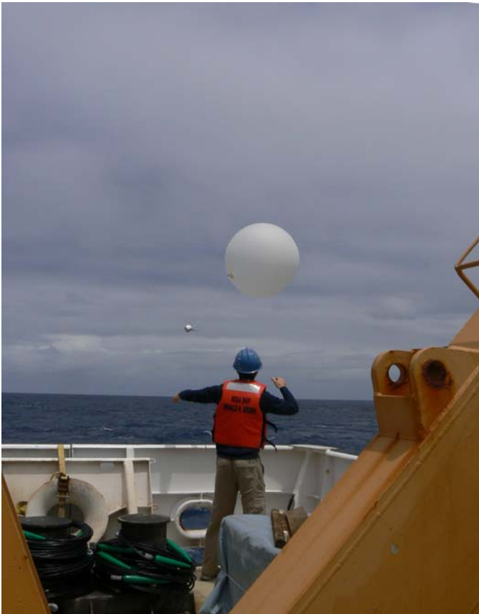
Figure 8. Photograph of a rawinsonde launch on October 25.
