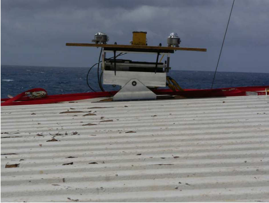
Figure 7. Photograph of PSD pitch/roll stabilized platform for solar and IR radiometer sensors in operation on its first field deployment. The system is mounted on top of a seatainer. The roll of the ship is apparent as the tilt relative to the horizon. Note the platform remains aligned with the horizon. A Kipp&Zonen pyrgeometer is on the left and an pyranometer on the right. The goldish cube in the center is the pitch/roll sensor.
