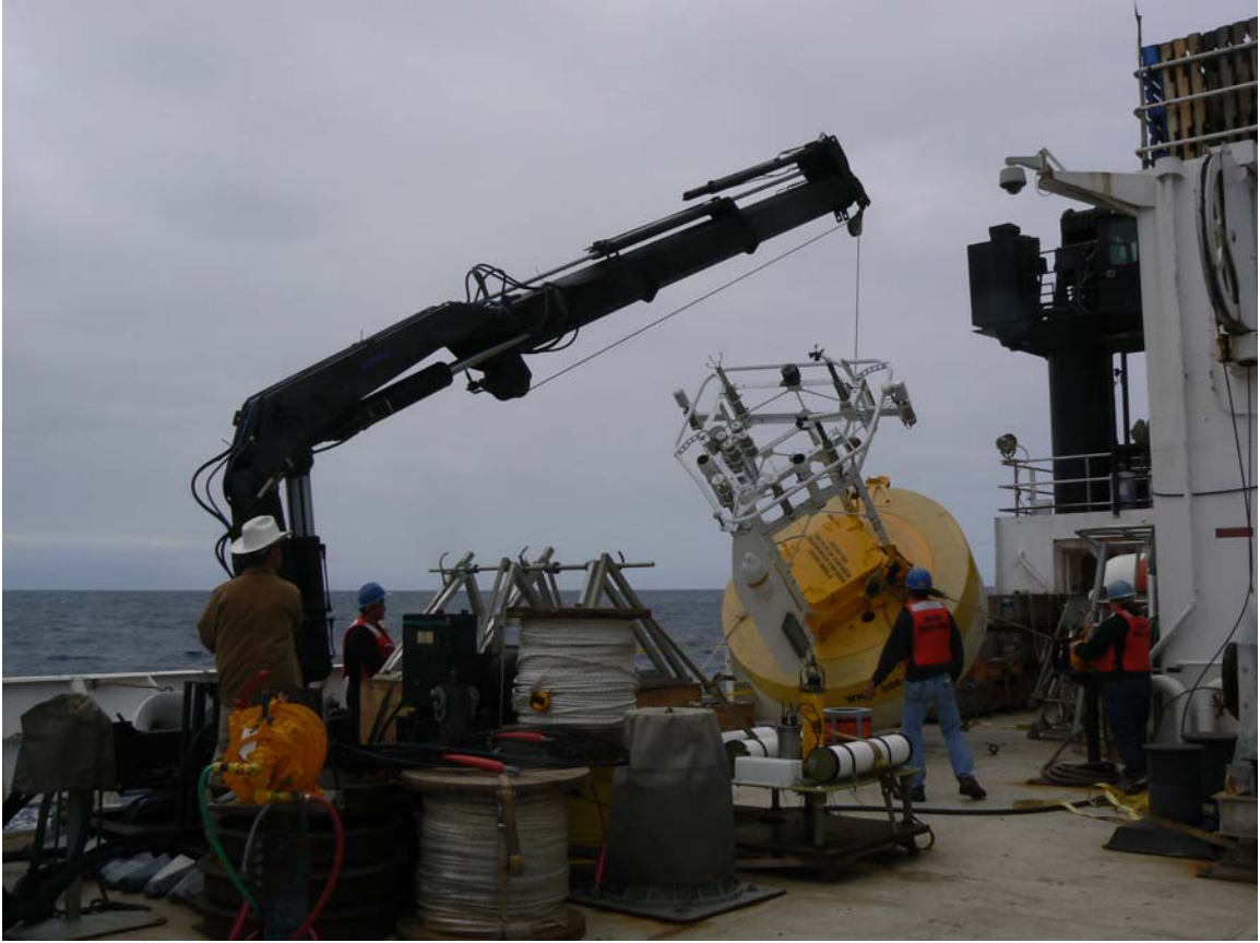
Figure 7. Photograph of WHOI buoy being position prior to launch on the aft deck of the Ronald H. Brown .
