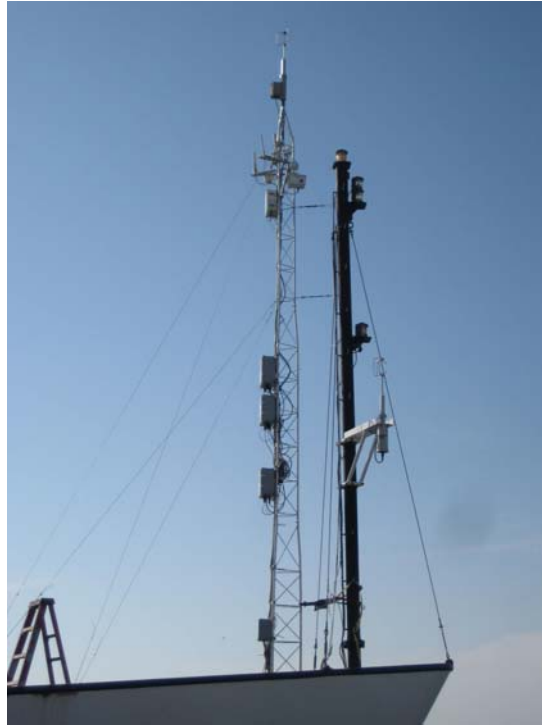
Figure 2. Views of the jackstaff and the PSD flux tower deployed on the R/V Moana Wave during STRATUS 2011.
