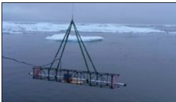
SIMS (Sea Ice Measurement System) suspended from port crane
