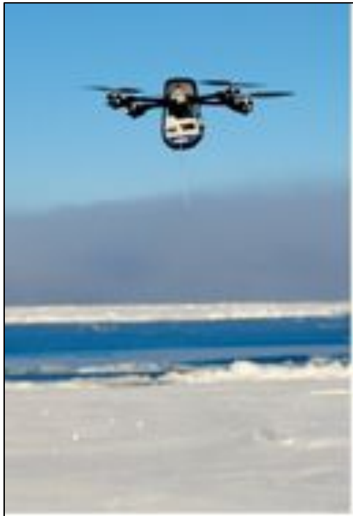
InstantEye UAS with radiosonde attached below
