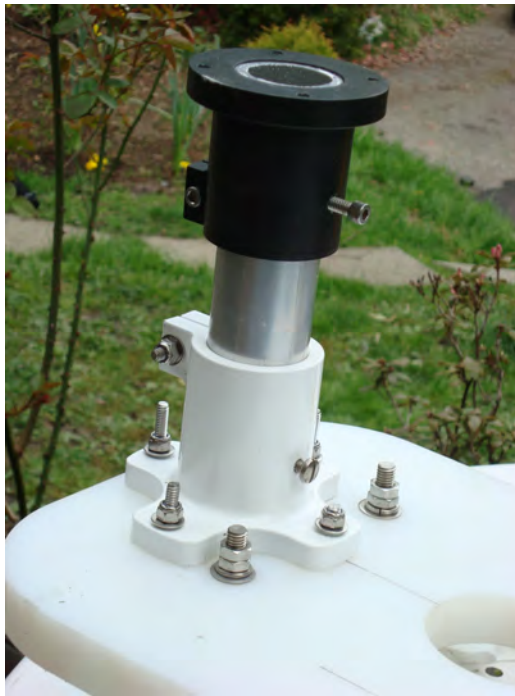
Figure 19: Two different pipe mount fittings are available for 1.5" schedule 40/80 pipe. The top pipe mount bracket is made of heavy duty plastic. It's fittings are threaded with helicoil inserts. The bottom fitting is 6061-T6 aluminum with thermoplastic powder coat.
