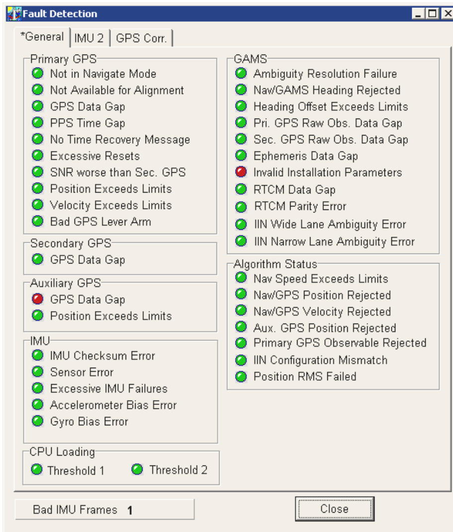
Figure 34: POSView Fault Detection
