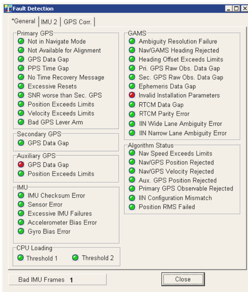
Figure 46: POSView Fault Detection
