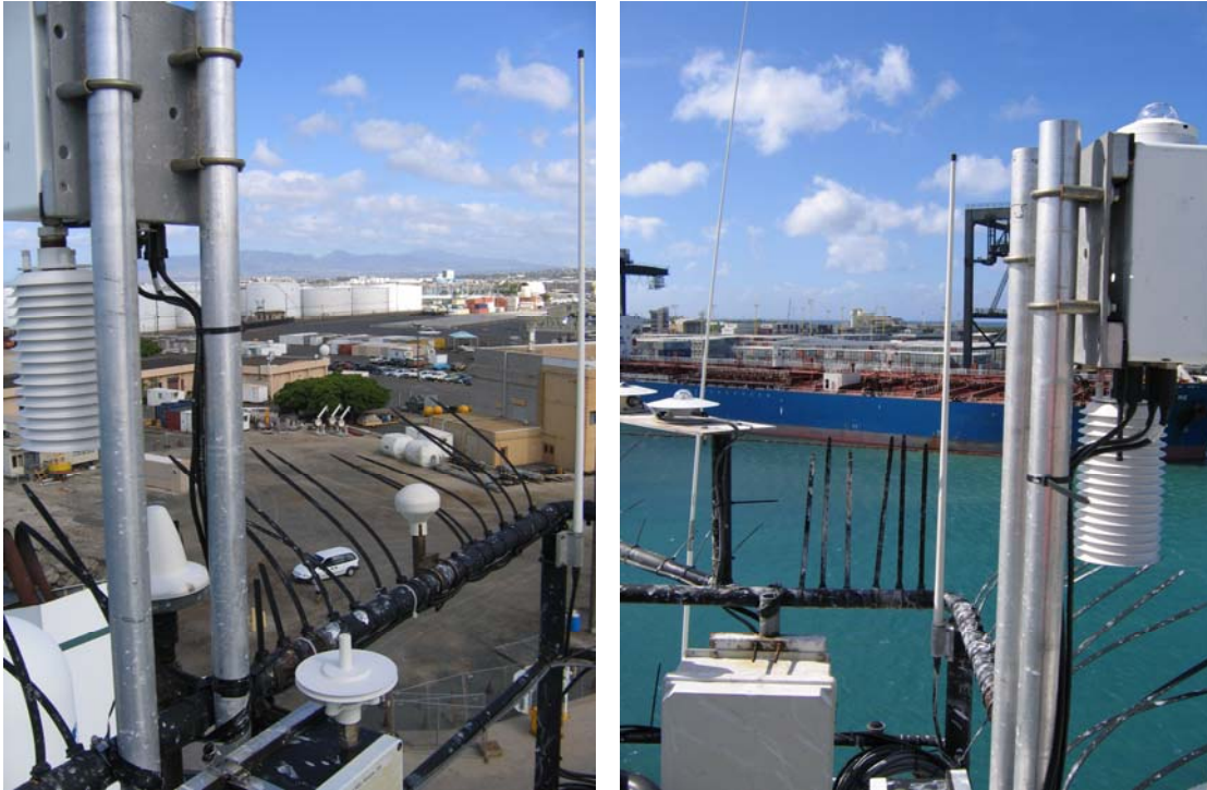
Figure A 2. Left: portside back view from the KM mast (AutoIMET pressure, T/RH sensors). Right: starboard back view from the KM mast (AutoIMET radiometers, and T/RH unit).
