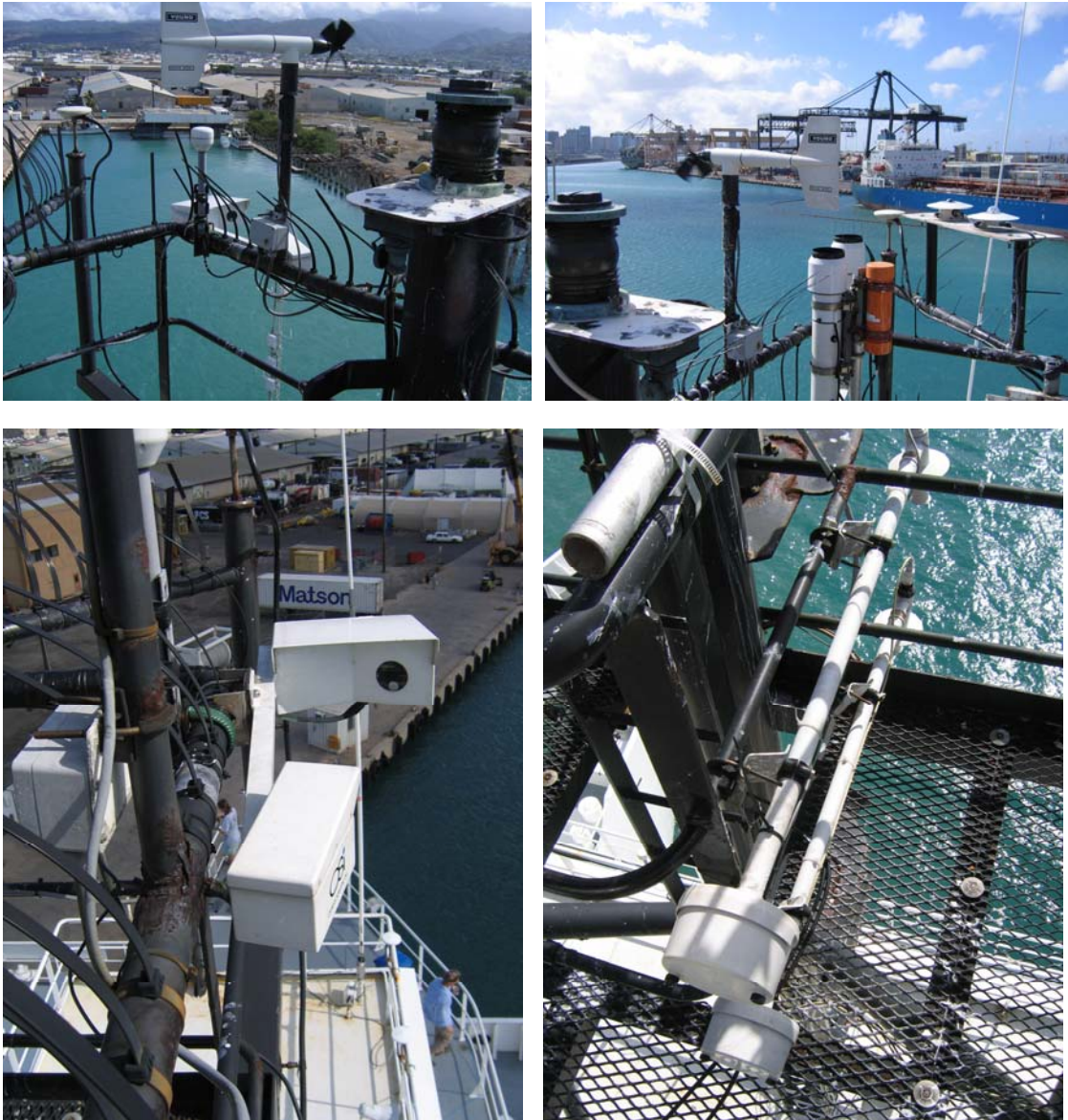
Figure A 1. Top left: portside view from the KM mast (anemometer, optical rain gauge). Top right: starboard view from the KM mast (anemometer, siphon rain gauge, radiometers). Bottom left: close-up view of the portside optical rain gauge. Bottom right: downward close-up view on the Rotronics T/RH unit, and the RTD air temperature sensor.
