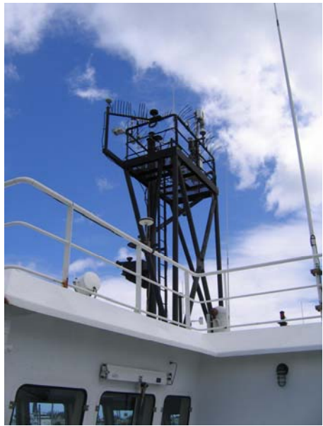
Figure 5. Instrument mast on top of the wheelhouse of the Kilo Moana.
