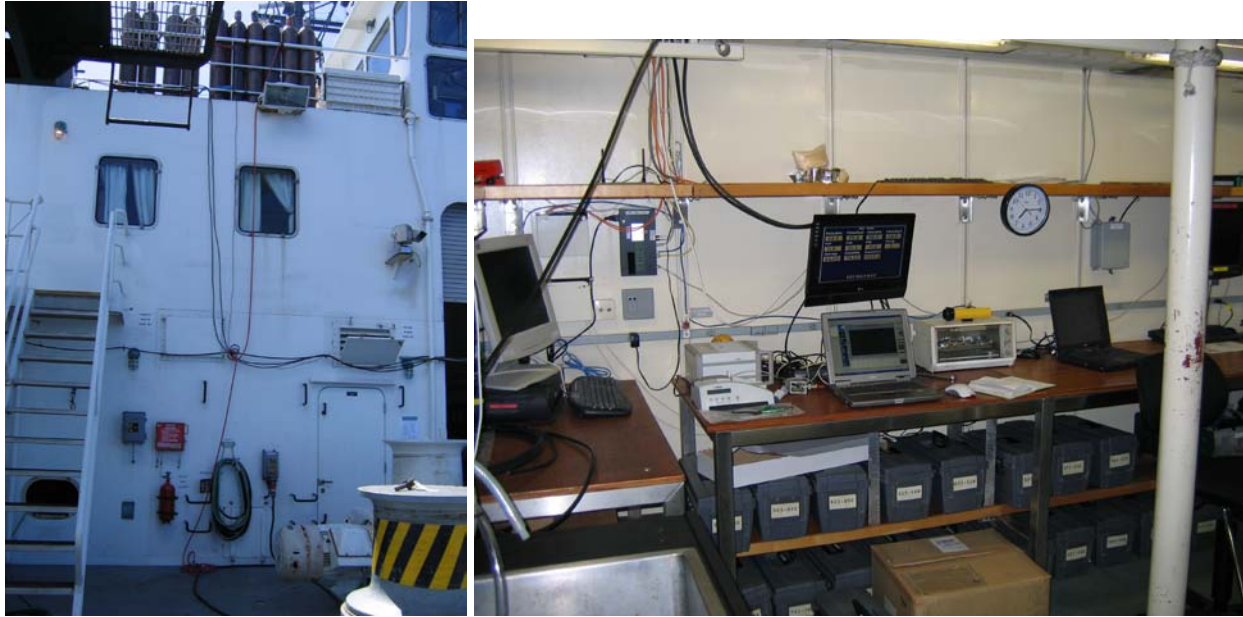
Fig.5. Left panel: view of the inflation site on the main deck with the Helium bottles on the 02 deck. Right panel: Vaisala radiosonde system deployed in Lab#1 of the Main deck.
