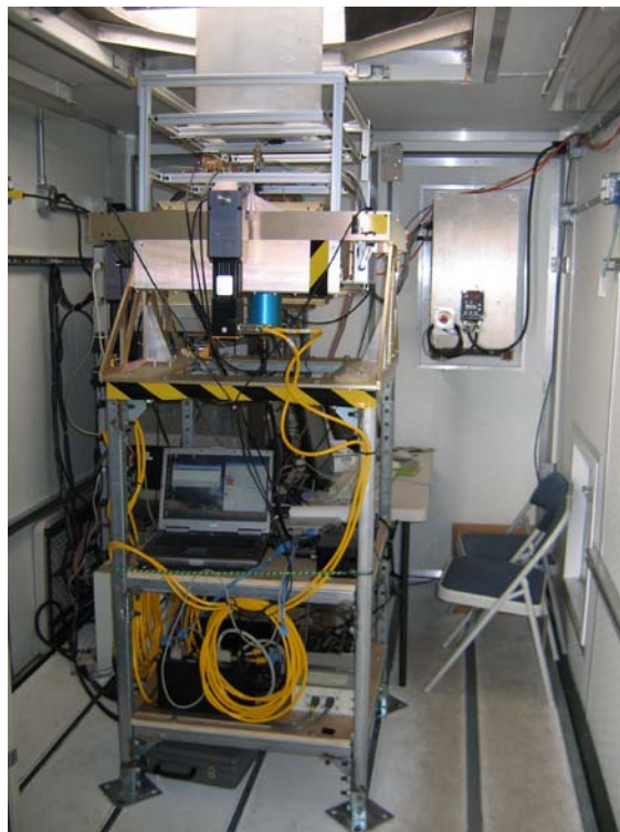
Fig.4. View of the W-band radar inside the operation van.
