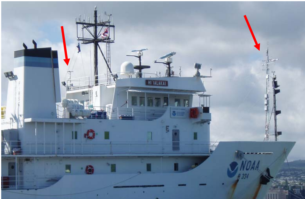
Figure 2. View of the flux tower and of the radiometers deployed on the R/V Hi'ialakai (red arrows).
