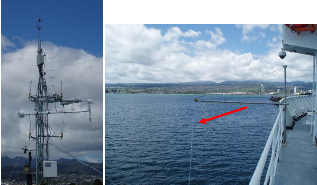
Figure 3. Left: Close-up view of the tower and its instruments. Right: Portside view of the 'sea snake' deployment (red arrow).
