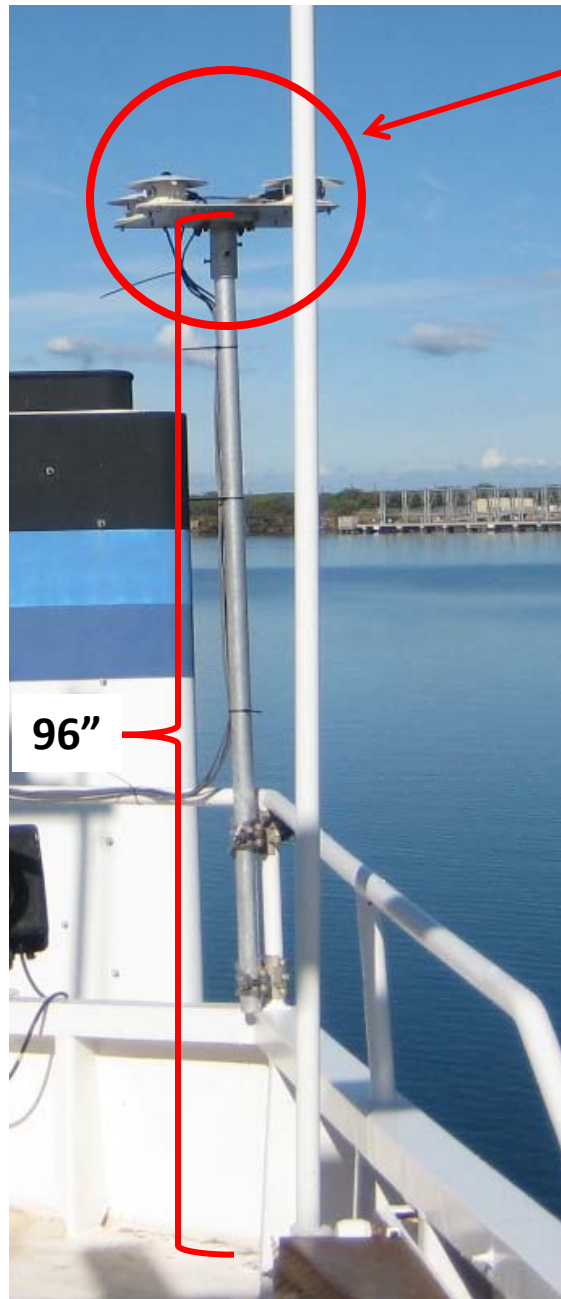
PSD3 radiometers 15.937m above water
