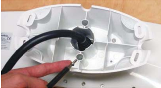
Figure 1-10. Fastening the fixed base to the Crescent V100
