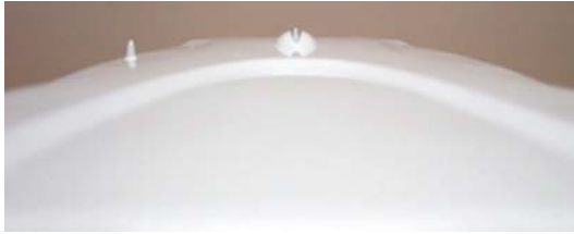
Figure 1-2. Correctly lined-up alignment sight
