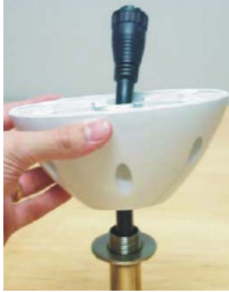
Figure 1-16. Completed cable run
