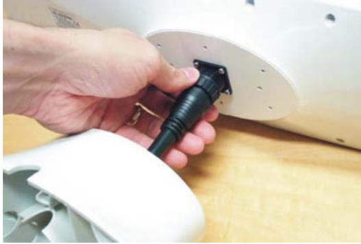
Figure 1-9. Connecting the power/data connector to Crescent V100
