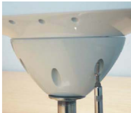
Figure 1-21. Fastening the pole base to the Crescent V100
