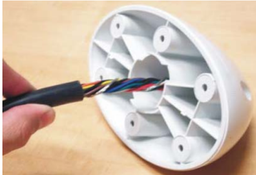
Figure 1-13. Running cable through the pole base
