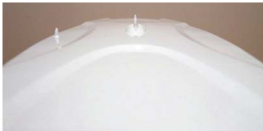
Figure 1-1. Lining up the alignment sight
