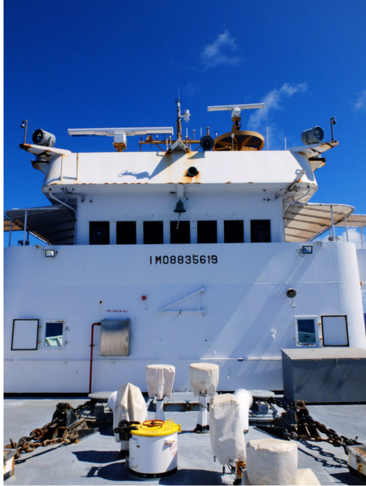
Ship T/RH and sonic anemometer on short mast at bridge roof centerline.
