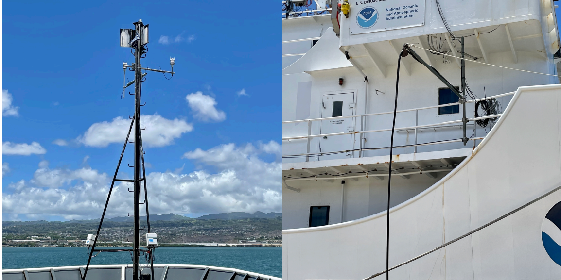
Figures 4-5: Bow installation for two WXT weather stations; starboard sea snake boom.
