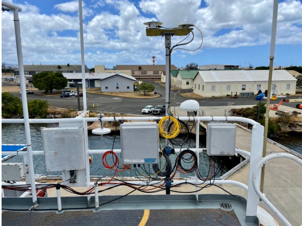
Figure 1: Radiometer mount, logger/pressure sensor box and ethernet switch box mounted to starboard railing on the pilot house roof.
